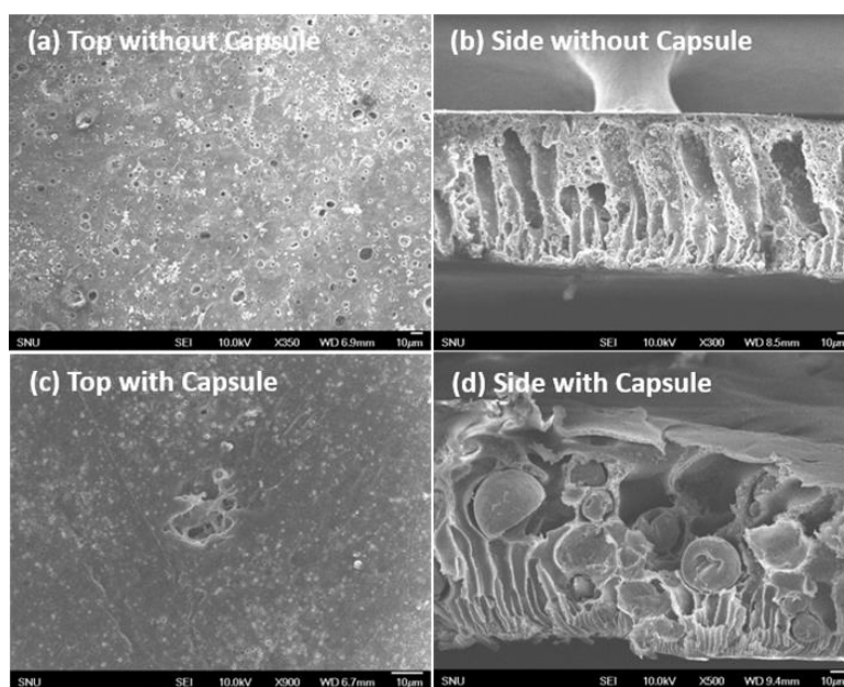
Figure 7. SEM images of pristine (a, b) and microcapsule (prepared with 3.0 g TDI, 2.0 g MDI, 4.5 g GA and 0.1 g DTAB) embedded (c, d) PES membranes cast by a phase inversion.
