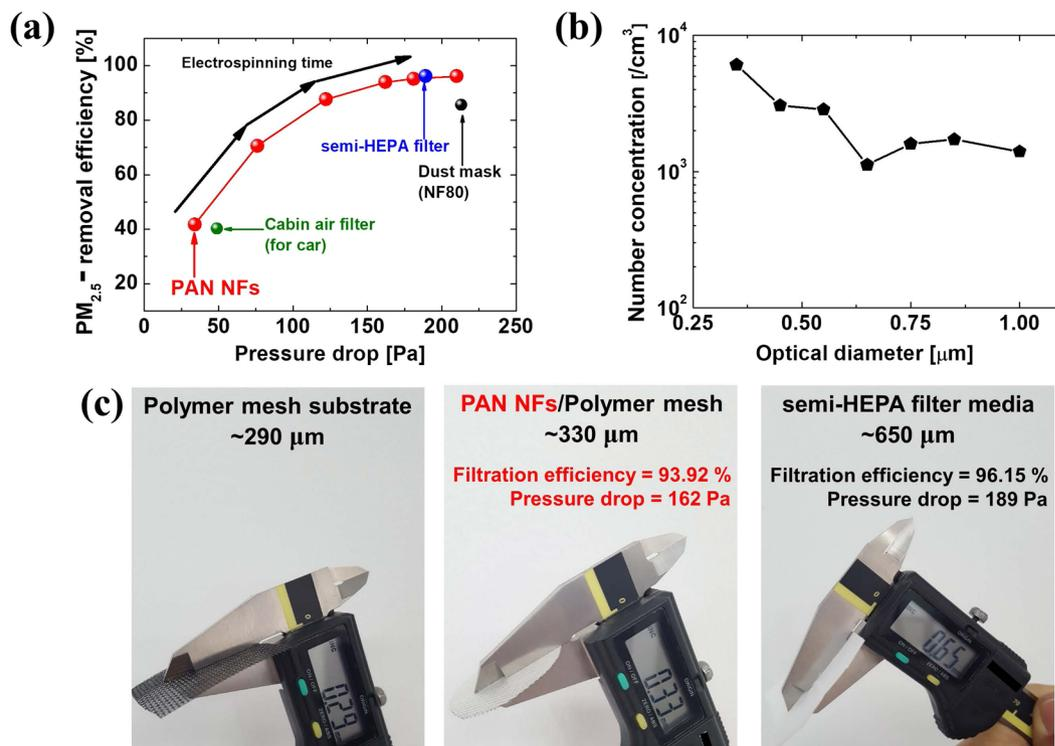
**Figure 2.** (a) Comparison of PM<sub>2.5</sub>-removal efficiency and pressure drop across PAN-NF filter medium and commercial filters (semi-HEPA filter, dust mask, and car cabin filter). (b) Size distribution of incense smoke particles as PM<sub>2.5</sub> source. (c) Comparison of the thickness of PAN-NF filter and semi-HEPA filter.
