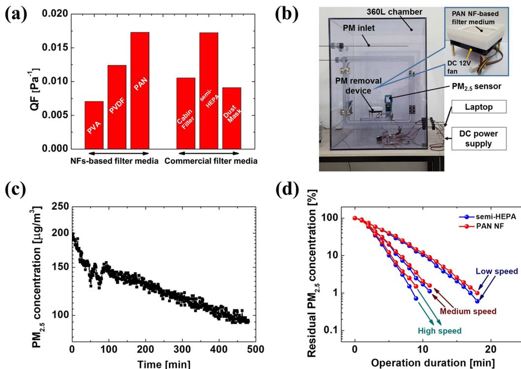
**Figure 3.** (a) Calculation results of quality factor (QF) for all air filters. (b) Photo of PM-removal test chamber and (inset) filtration device. (c) Change in PM<sub>2.5</sub> concentration in a closed chamber without a PM-removal device. (d) Comparison of the PM<sub>2.5</sub>-removal performance of a PAN-NF-based filter and a semi-HEPA filter.
