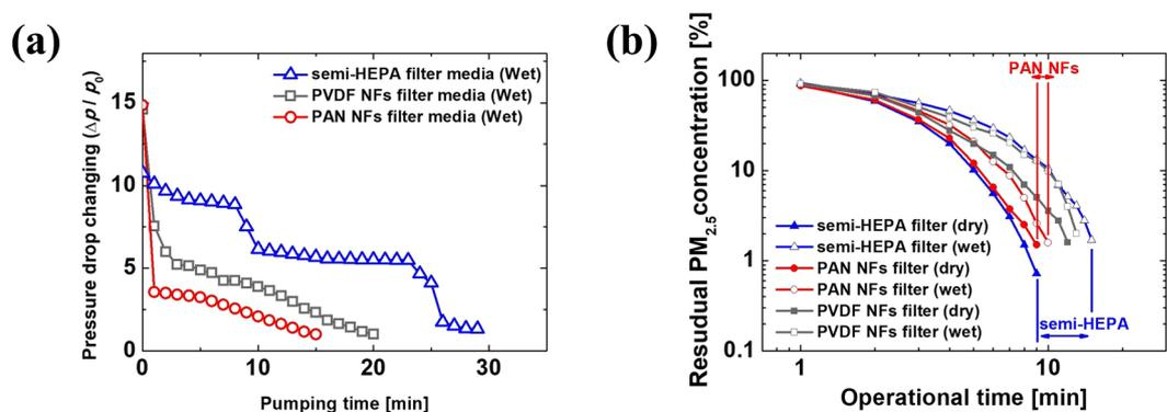
**Figure 5.** (a) Changes in pressure drop cross semi-HEPA filter medium, PVDF-NF filter medium, and PAN-NF filter medium as a result of water absorption. (b)  $PM_{2.5}$ -removal performance of the semi-HEPA, PVDF-NF, and PAN-NF filter media under dry and wet conditions.
