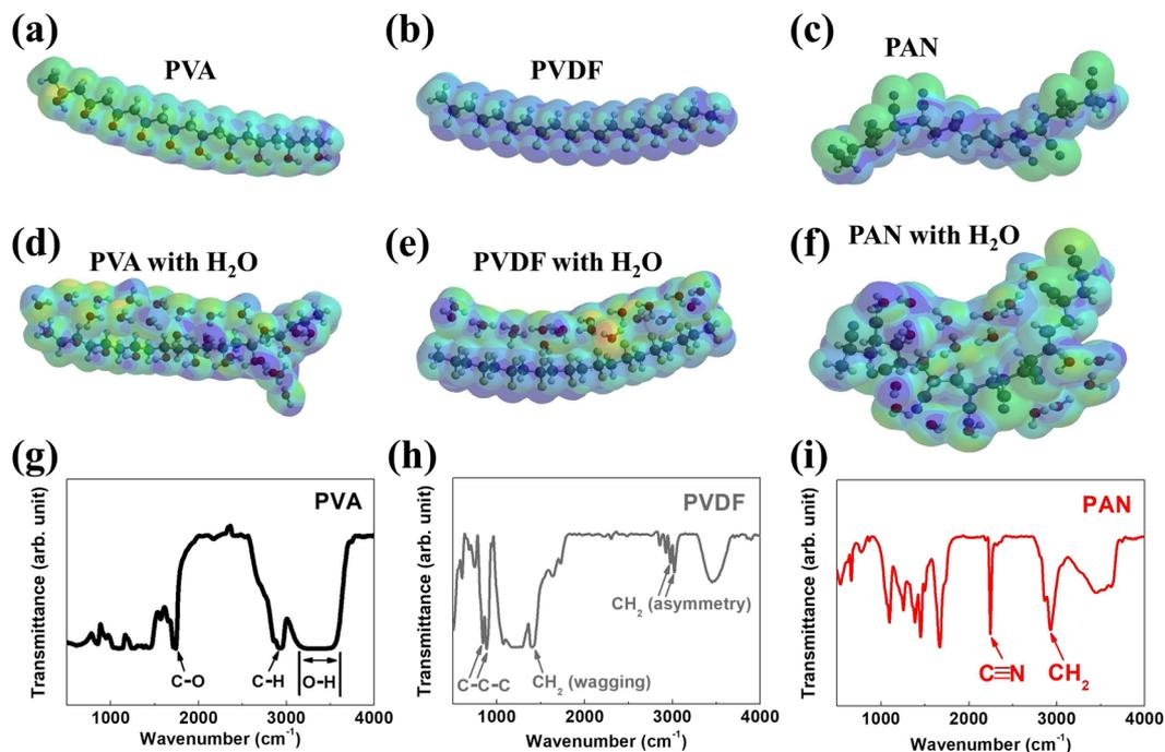
**Figure 1.** DFT calculation results for (a) 2 nm linear PVA molecule without H<sub>2</sub>O, (b) 2 nm linear PVDF molecule without H<sub>2</sub>O, (c) 2 nm twisted PAN molecule without H<sub>2</sub>O, (d) 2 nm PVA molecule with 20 H<sub>2</sub>O molecules, (e) 2 nm PVDF molecule with 20 H<sub>2</sub>O molecules, and (f) 2 nm PAN molecule with 20 H<sub>2</sub>O molecules. FTIR results for (g) PVA-NF filter medium, (h) PVDF-NF filter medium, and (i) PAN-NF filter medium.
