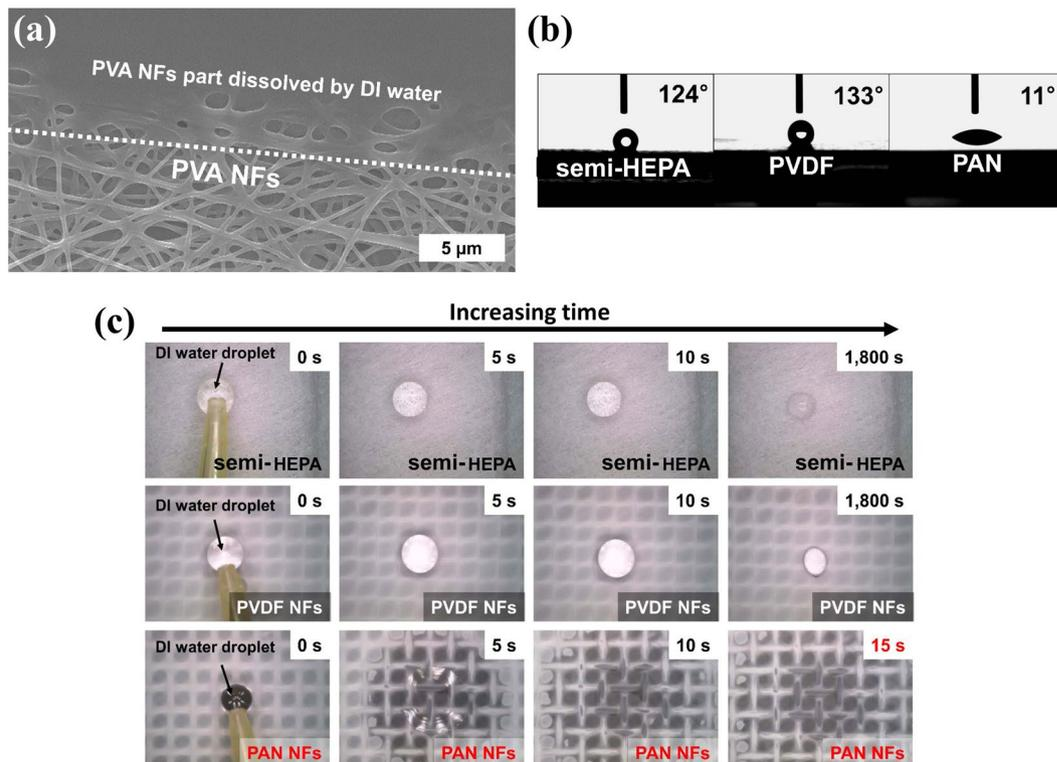
**Figure 4.** (a) Dissolution of PAN NFs by DI water. (b) Contact angle of DI water on the surface of semi-HEPA filter medium, PVDF-NF medium, and PAN-NF filter medium. (c) Behavior of DI water droplet on the surface of semi-HEPA filter medium, PVDF-NF filter medium, and PAN-NF filter medium.
